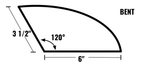
SUITABLE FOR FRAMES WITH GUSSETED BRACES AT SEAT TUBE, STEEPLY ANGLED SEAT TUBES, OR BIKES WITH MINIMAL EXPOSED SEAT POST.
